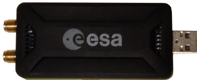
Figure 2.43: LimeSDR Mini transceiver.
