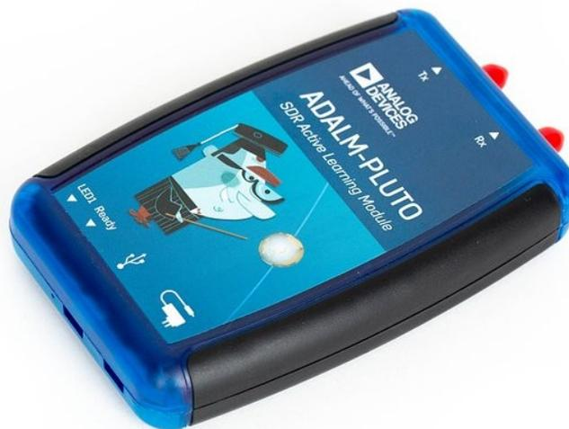
Figure 2.121: The Analog Devices PlutoSDR transceiver.
