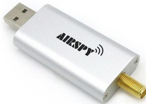
Figure 2.26: The Airspy Mini receiver.
